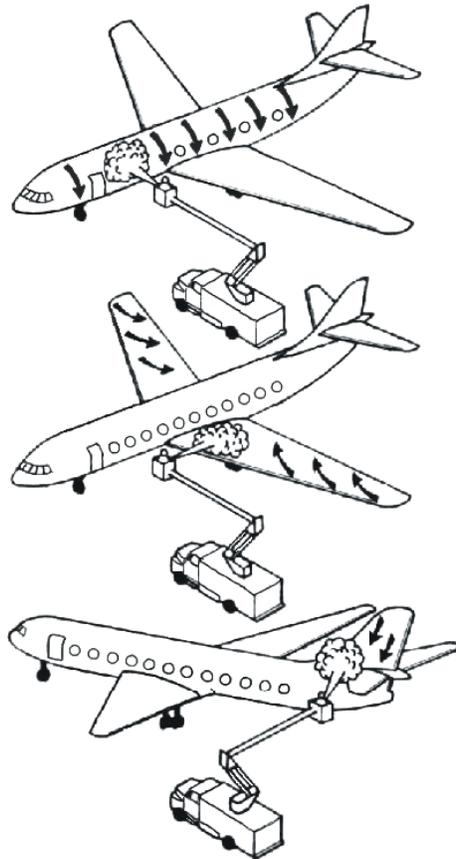
**Figure 1. Systematic and symmetrical de-icing of aircraft.**
